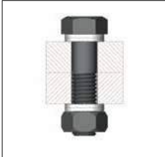
Hexagon bolt in a through hole secured on both sides
