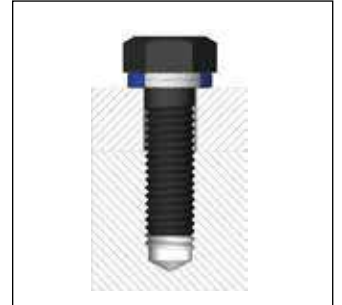
Hexagon bolt secured in a blind hole
