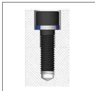
Countersunk socket head bolt secured in position
