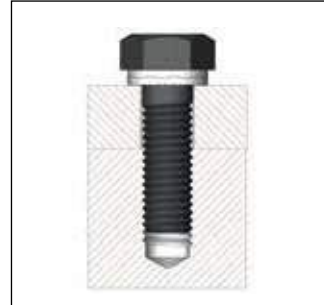
Hexagon bolt secured in a blind hole
