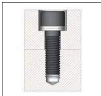
Countersunk socket head bolt secured in position
