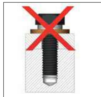
No locking function in combination with flat washers
