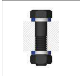
Hexagon bolt in a through hole secured on both sides
